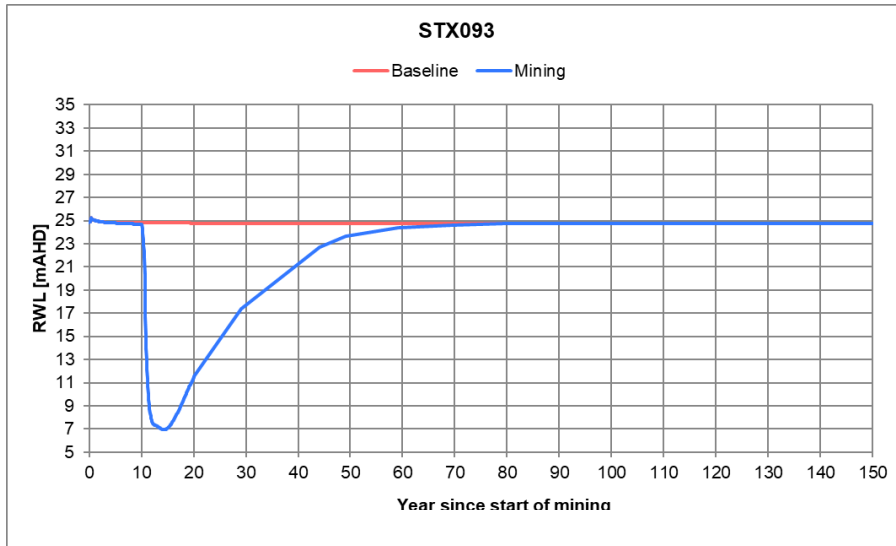
Figure 16-118 Hydrograph showing predicted transient water table response to mine water affecting activities at STX 093 (stygo fauna bore, Type 1 GDE)
